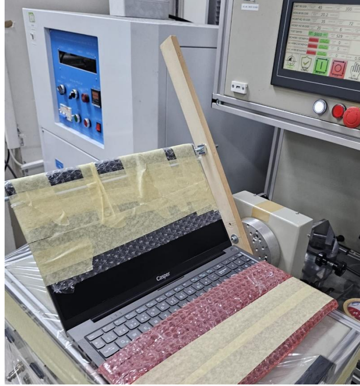
Photo 7. Hinge durability test of the Notebook
