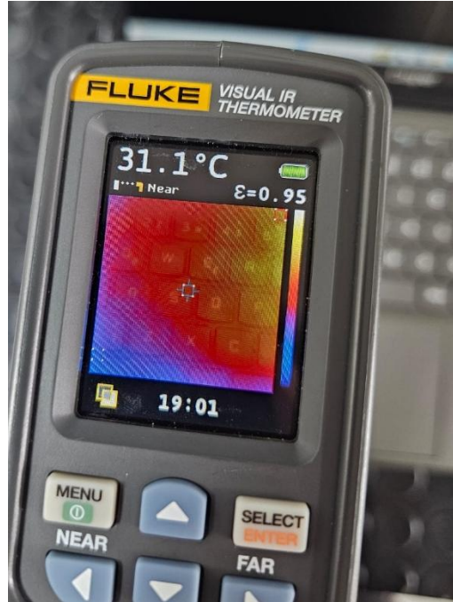
Photo 4. Thermal performance test of the Notebook
