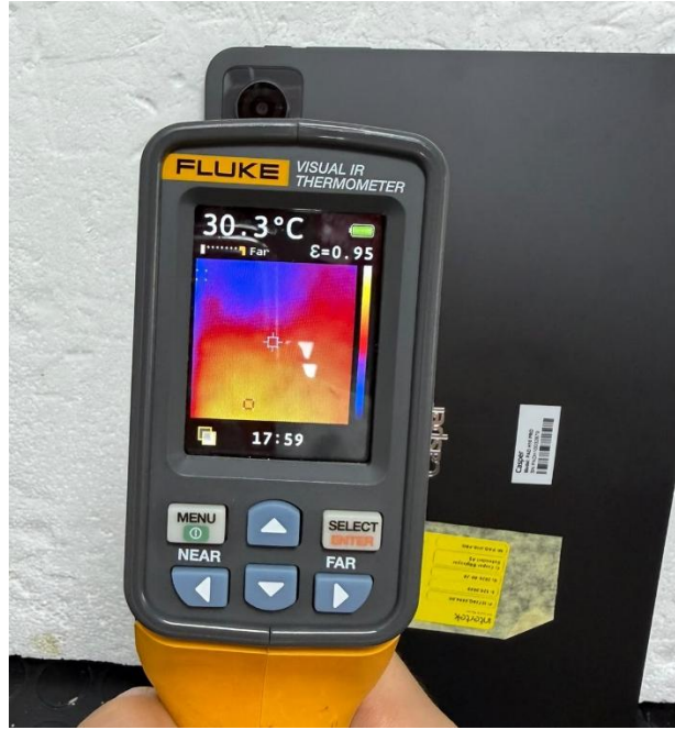
Photo 4. Thermal performance test of the Tablet
